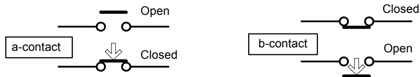
Fig. 9- 7 The operation diagram of a-contact and b-contact
