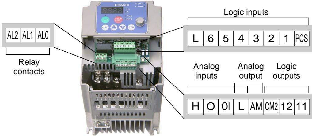
Specifications for the logic connection terminals are in the following table:
