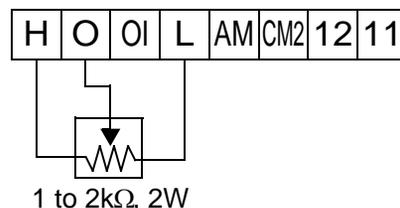
**Voltage Input** – The voltage input circuit uses terminals [L] and [O]. Attach the signal cable’s shield wire only to terminal [L] on the inverter. Maintain the voltage within specifications (do not apply negative voltage).
