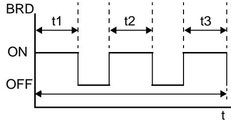
$$\boxed{\text{B } 90} \quad T\% = \frac{(t1 + t2 + t3)}{100 \text{ seconds}} \times 100$$
