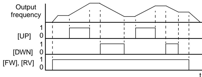
It is possible for the inverter to retain the frequency set from the [UP] and [DWN] terminals through a power loss. Parameter C101 enables/disables the memory. If disabled, the inverter retains the last frequency before an UP/DWN adjustment. Use the [UDC] terminal to clear the memory and return to the original set output frequency.
