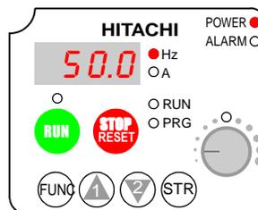
For the powerup test, monitor the motor speed indirectly by viewing the inverter's output frequency. The *output frequency* must not be confused with *base frequency* (50/
