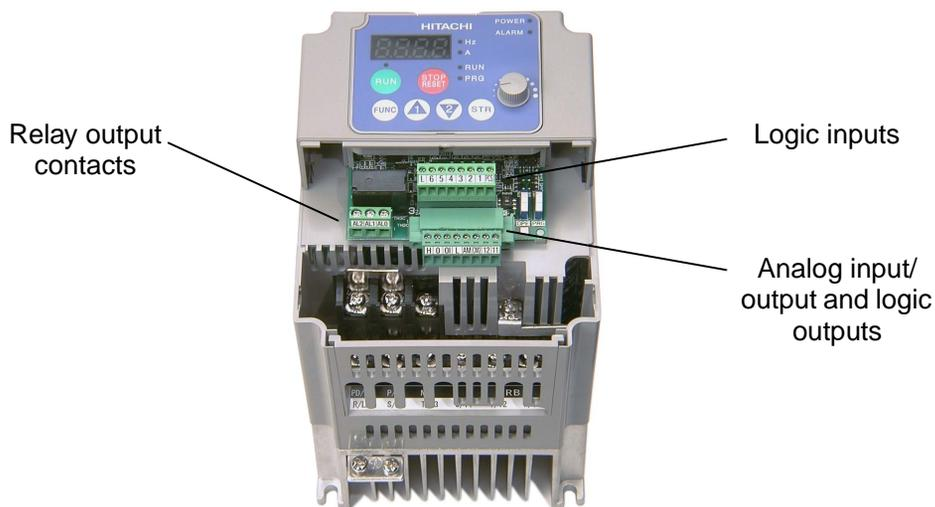
**Logic Connector Removal/Replacement** - The two 8-position main logic connectors are removable from the circuit board to make testing or service more convenient. Note that the relay output connector is not removable, as it must carry higher currents and provide high integrity for alarm conditions. The alarm circuit may carry hazardous live voltages (from external wiring) even when the main power to the inverter is OFF. So, never directly touch any terminal or circuit component.
