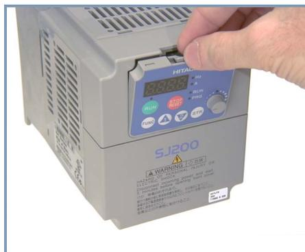
**Internal LED Indicators / Communications Connector** - Refer to the keypad bay in the illustration below. After removing the keypad, the internal LED viewing window will be visible. These LEDs indicate status for your convenience when the keypad is remotely mounted and you are nearer to the inverter location.
