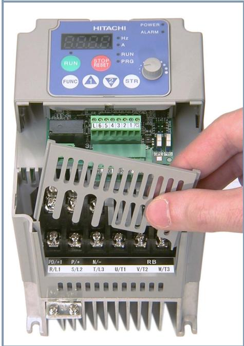
The power input and motor 3-phase wiring connect to the lower row of terminals. The upper row of power terminals connect to optional dynamic braking components.
