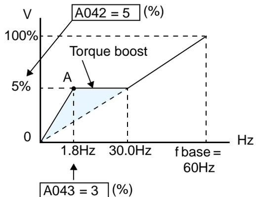
breakpoint of the boost (point A on the graph) by using parameters A042 and A043. The manual boost is calculated as an addition to the standard V/f curve.
