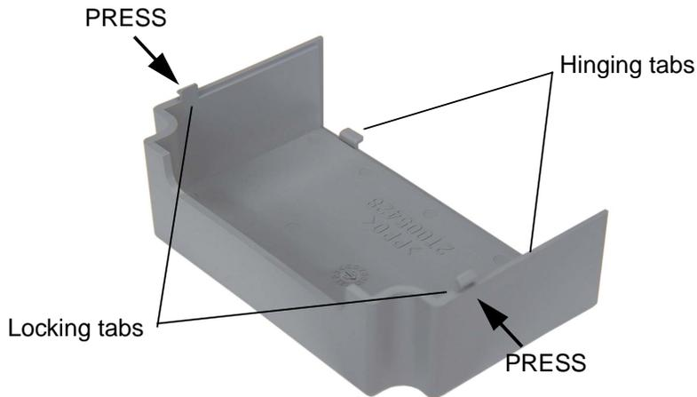
The figure below shows the procedure for removing the housing cover. While pressing inward on the housing, it is helpful to wiggle the cover side-to-side in order to release the locking tabs. **DO NOT** force the cover open; it is possible to break a tab in this way.
