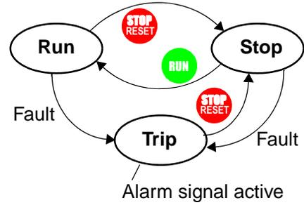
We must make a distinction between the alarm signal AL and the alarm relay contacts [AL0], [AL1] and [AL2]. The signal AL is a logic function, which you can assign to the open collector output terminals [11] or [12] or the relay outputs.
