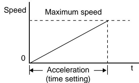
However, the slope is constant, corresponding to the full-scale accel or decel time setting. For example, the full-scale acceleration setting (time) may be 10 seconds—the time required to go from 0 to 60 Hz.
