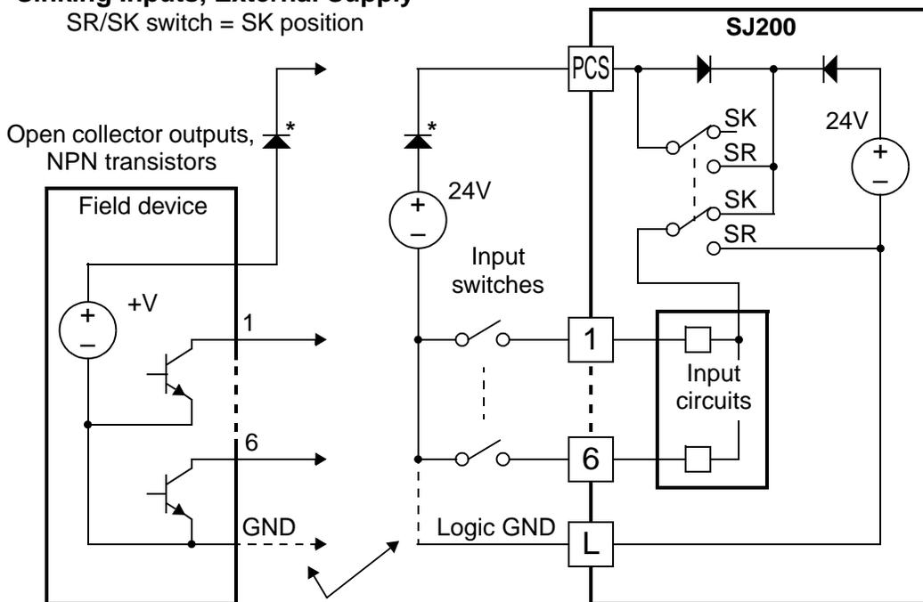
\* Note: If the external power supply GND is (optionally) connected to [L], then install the above diode.
