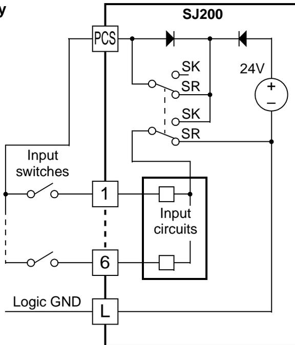
The two diagrams below show input wiring circuits using an external supply. If using the upper wiring diagram, be sure to use a diode with the external supply. This will prevent a power supply contention in case the SR/SK switch is accidentally placed in the incorrect position. Be sure to use the correct SR/SK switch position shown for each wiring diagram.
