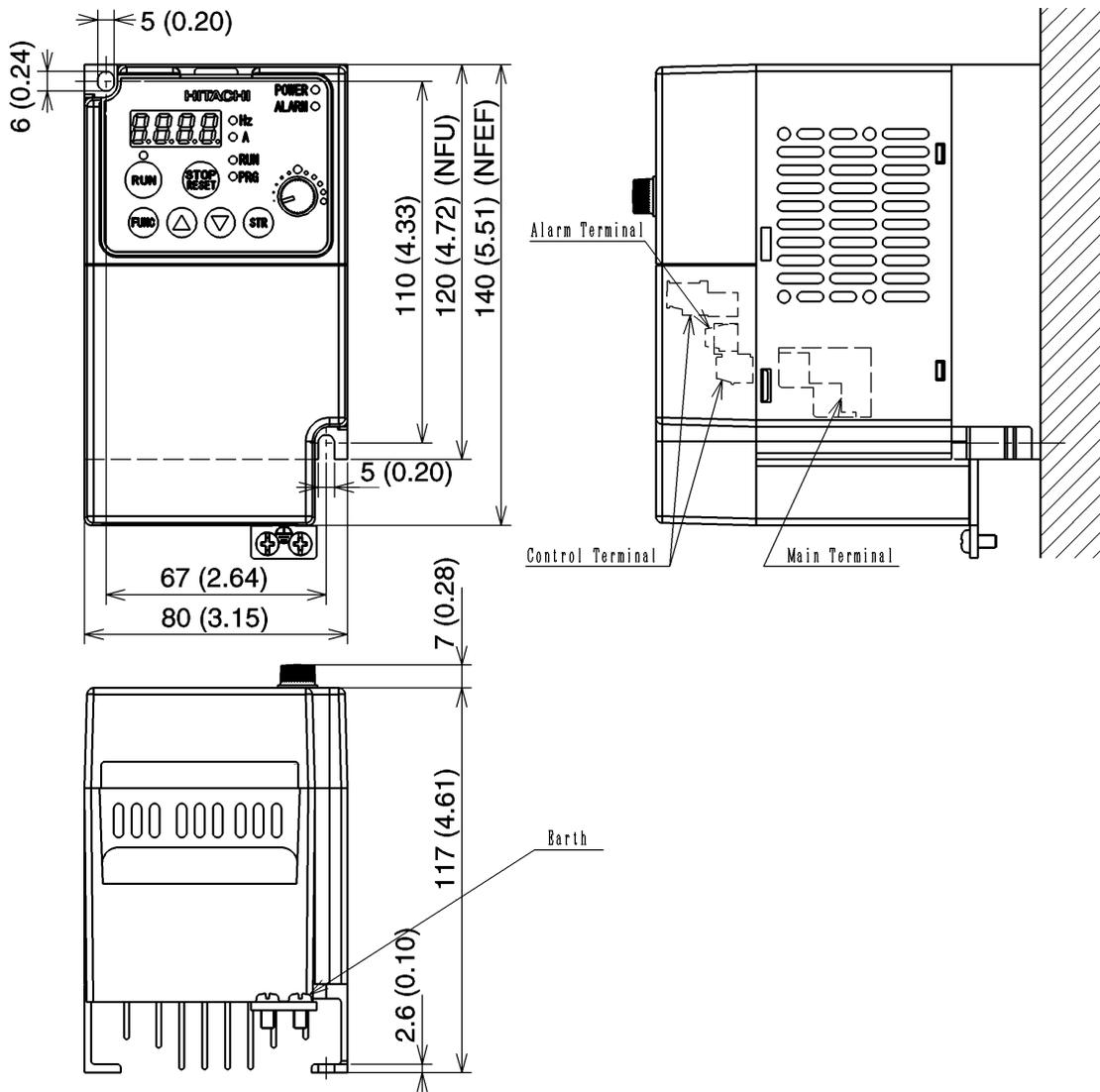
Inverter Mounting and Installation
