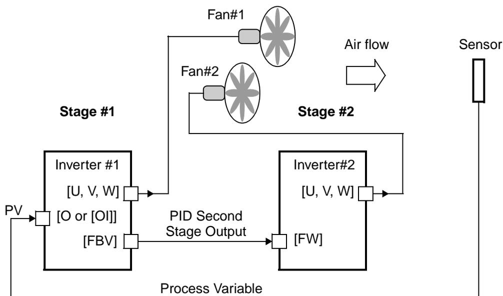
To use the PID Second Stage Output feature, you will need to choose upper and lower limits for the PV, via C053 and C052 respectively. As the timing diagram below shows, these are the thresholds Stage #1 inverter uses to turn ON or OFF Stage #2 inverter via the [FBV] output. The vertical axis units are percent (%) for the PID setpoint, and for the upper and lower limits. The output frequency, in Hz, is superimposed onto the same diagram.
