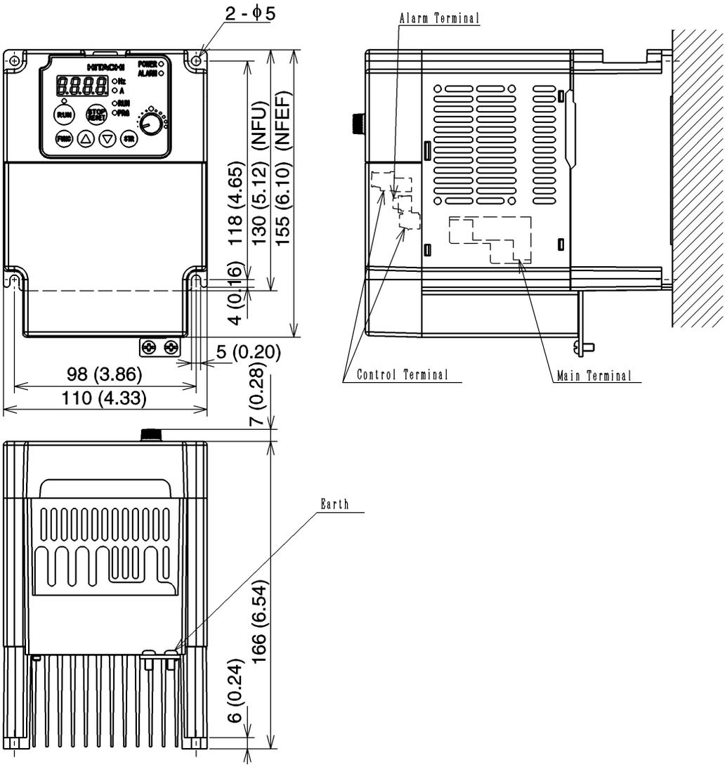
Inverter Mounting and Installation
