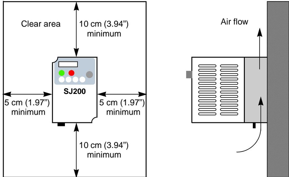
Inverter Mounting and Installation
