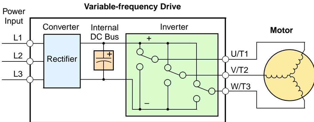
The simplified drawing of the inverter shows three double-throw switches. In Hitachi inverters, the switches are actually IGBTs (insulated gate bipolar transistors). Using a commutation algorithm, the microprocessor in the drive switches the IGBTs on and off at a very high speed to create the desired output waveforms. The inductance of the motor windings helps smooth out the pulses.
