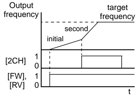
In the graph shown above, the [2CH] becomes active during the initial acceleration. This causes the inverter to switch from using acceleration 1 (F002) to acceleration 2 (A092).
