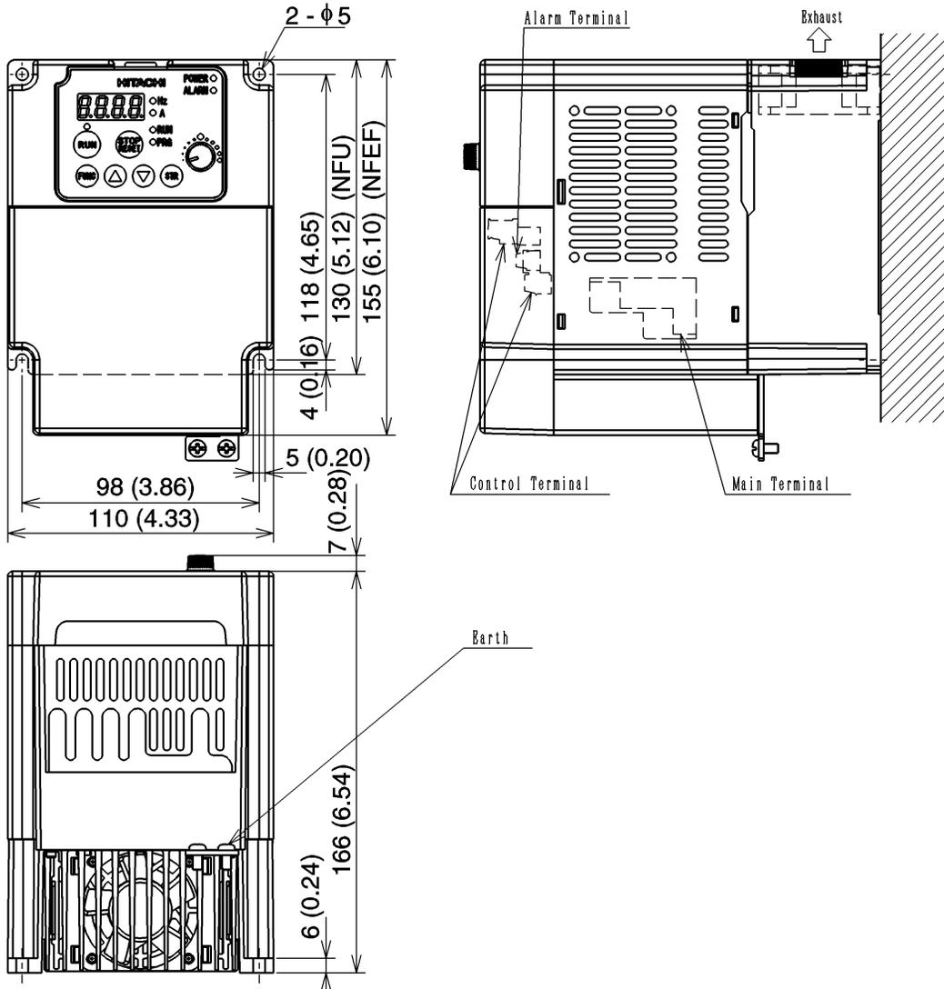
Inverter Mounting and Installation
