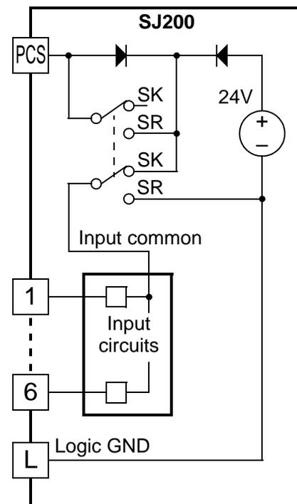
The two diagrams below show input wiring circuits using the inverter's internal +24V supply. Each diagram shows the connection for simple switches, or for a field device with transistor outputs. Note that in the lower diagram, it is necessary to connect terminal [L] only when using the field device with transistors. Be sure to use the correct SR/SK switch position shown for each wiring diagram.
