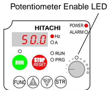
If the Potentiometer Enable LED is OFF, follow the steps below.
