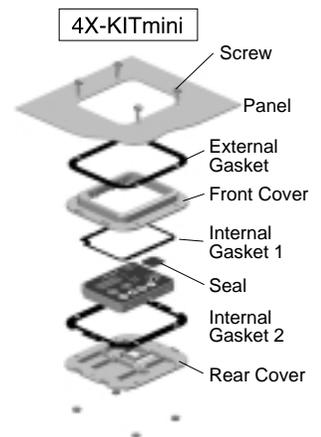
You can mount the keypad with the potentiometer for a NEMA1 rated installation. The kit also provides for removing the potentiometer knob to meet NEMA 4X requirements, as shown (part no.4X-KITmini).
