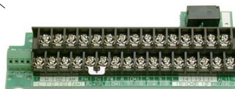
Control Signal Terminal Block (See Chapter 4 for wiring)
