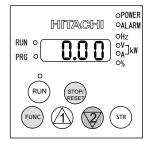
3) When the initialization is completed, the monitor displays data "0.00". (In case of b038 = 001) Confirm that the settings have been initialized.
