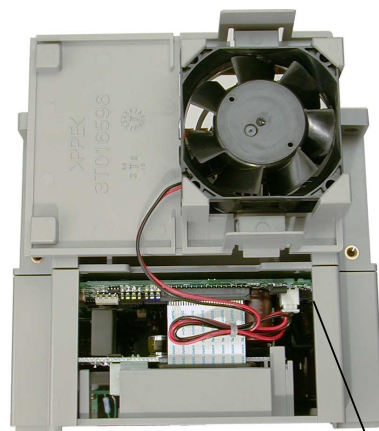
PWB connector for fan assembly wiring
