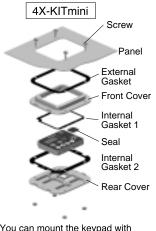
You can mount the keypad with the potentiometer for a NEMA1 rated installation. The kit also provides for removing the potentiometer knob to meet NEMA 4X requirements, as shown (part no.4X-KITmini).
