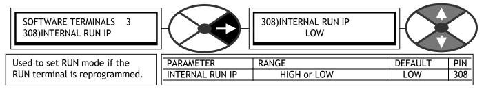
The RUN command normally comes from the default RUN terminal (T31) and will show the state of T31. However this terminal may be used as a programmable terminal in the event of a shortage of digital inputs. In this case 308)INTERNAL RUN IP must be disconnected from the RUN terminal and set HIGH to allow the drive to run.
