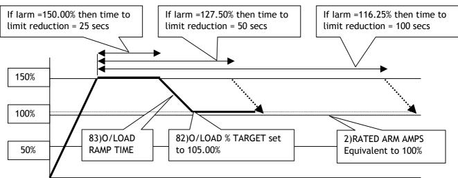
6.8.3.1.1 Diagram showing O/LOAD % TARGET set to 105%
