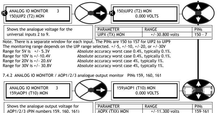
Note. The analogue output monitor for AOP1/2/3 shows the value written to that output. If the output is overloaded or shorted then the value shown will not agree with the actual output.
