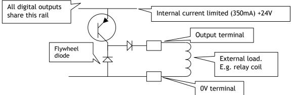
This shows the output configuration for each digital output DOP1 to DOP3 and DIO1 to DIO4
