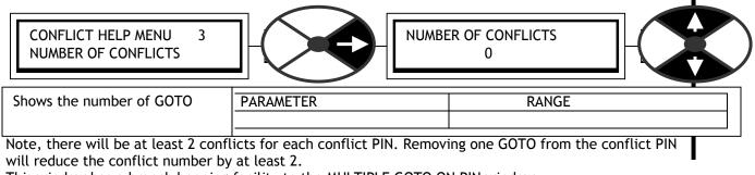
This window has a branch hopping facility to the MULTIPLE GOTO ON PIN window.
