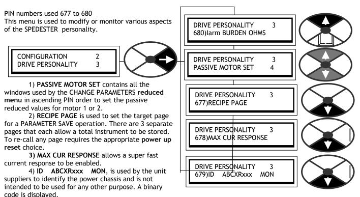
5) Jarm BURDEN OHMS is used, along with the actual burden, to derate the model armature current.
