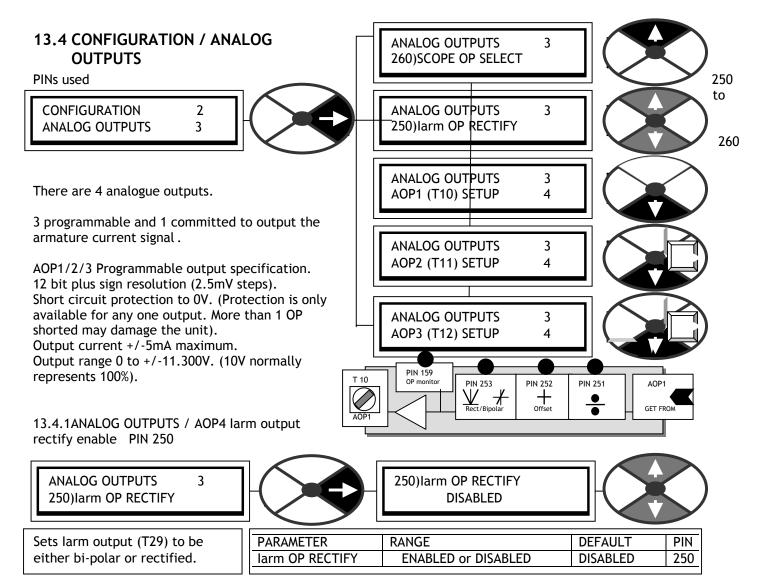
13.4.2ANALOG OUTPUTS / AOP1/2/3/4 SETUP
