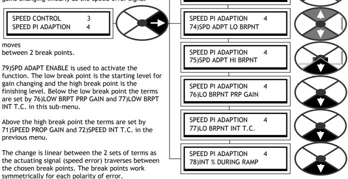
There is also the ability to prevent the integrator from accumulating error during a long speed up ramp. This can be useful for systems involving high inertias where there is a possibility of speed error at the top of the ramp while the loop removes the integrator error. See 6.2.16 RUN MODE RAMPS / Ramping flag PIN 35. See 6.7.7.7 SPEED PI ADAPTION / Using small speed inputs. The default gives low gain for small inputs.
