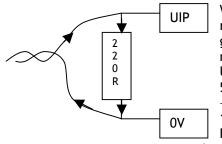
When using 4-20mA loop signals all that is required is to fit an external burden resistor of 220 Ohms between the input and 0V. The resulting voltage signal generated by passing the signal current through the burden will be +0.88V for 4 mA (represents 0%) and 4.4V for 20mA (represents 100%). Using the appropriate UIPX SETUP block, select the following :-
