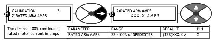
This current may be less than the value on the motor data-plate, but must not normally be higher. (However, see also 6.8.3.1.2 How to get overloads greater than 150% using 82)O/LOAD % TARGET).
