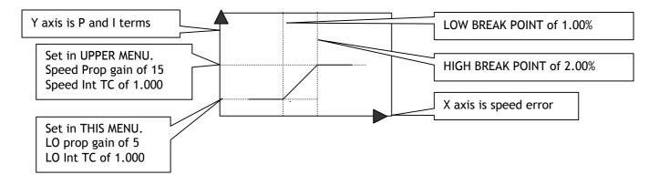
Note. The default settings are designed to give lower gain with low error. This provides smooth steady state performance. Applications that require precise control at very low speeds may function better with the adaption disabled.
