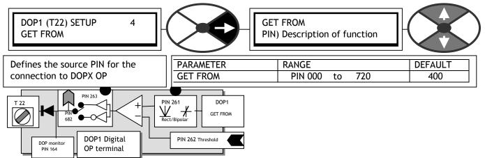
The connection is made here for the digital output block source. It may be a linear or logic value. After processing by the rectifier box it gets compared to the threshold. The comparator output state HIGH or LOW is then inverted or not inverted by the inverter mode box and becomes a 24V logic signal.
