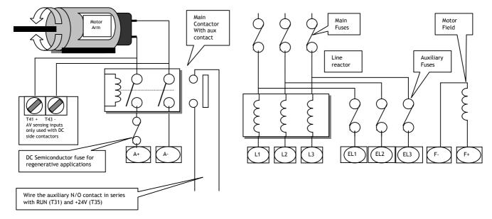
Advantages The auxiliary supplies are permanently energised. This allows the synchronisation circuits to lock onto the supply prior to the application of power to the motor. This results in a fast release of current to the armature because it avoids the synchronisation delay. Also the field can remain energised after contactor drop out allowing dynamic braking and/or condensation prevention in standby field mode.
