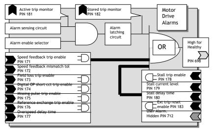
If an alarm is enabled, triggered and latched causing the drive to shut down, then after approximately a further 10mS no further alarms will be latched. Hence when the latched status of the alarms is monitored it is unlikely that more than 1 alarm will be latched. If however more than 1 is latched, then the first that arrived and initiated the shutdown can be determined from the DRIVE TRIP MESSAGE menu.
