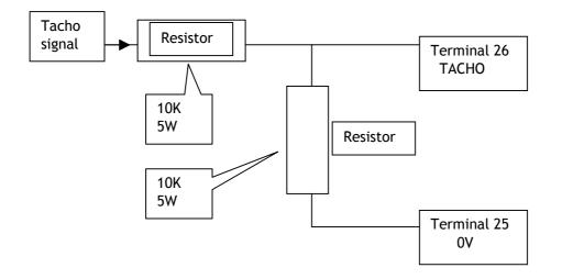
The network shown will allow full scale voltages up to 400 Volts. The number scrolled in the window should be set to half the full scale tacho volts. Appropriate measures must be taken to dissipate the heat from the dropper resistors. The total power in watts dissipated will be  $(Tacho signal volts)^2 / 20,000$ .
