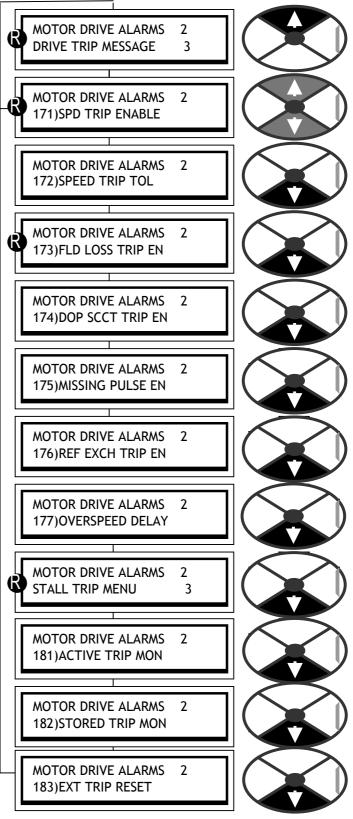
for the individual alarms. The quoted times are typical since the delay is implemented in microprocessor "cycle time" units which vary with microprocessor loading. The arrival of the alarms prior to the trigger can be accessed for advance warning purposes using the active monitor window. There is a USER ALARM on hidden PIN 712. This may be connected by the user to any flag, to trip the drive.
