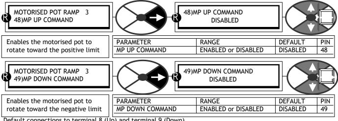
6.4.4 MOTORISED POT RAMP / MP Up / Down command PINs 48 / 49
