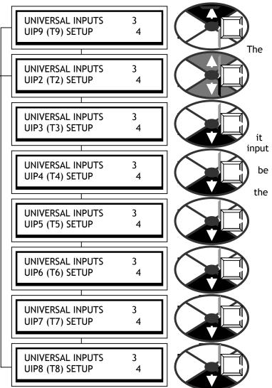
nullify the internal connection, (set 67)SPD/CUR RF3 RATIO in the SPEED REF SUMMER menu to 0.0000), then reconfigure the linear GOTO. The parameter 64)SPEED REF 3 MON is a monitor of the UIP3 analog output.
