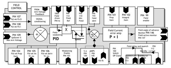
1) Voltage output clamp. This is an open loop setting of the field bridge-firing angle allowing the DC output voltage to be set between 0 to 90% of the incoming supply voltage. E. g. for an AC supply of 400V the 90% output voltage is 360V DC. Note if the AC supply varies, then the field output voltage will vary in proportion. Also if the field resistance changes then the resulting output current will change.
