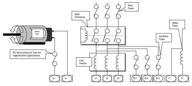
Advantages The field winding is electromechanically isolated by the main contactor. Some retro fit installations are only able to provide the 3 main phases because the main contactor is remotely located to the drive panel, in which case this wiring method may be preferred.
