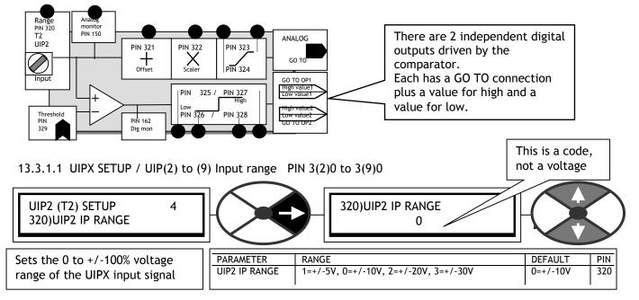
The +/-5V and +/-10V ranges are the most accurate (0.4%, typically 0.1%).
