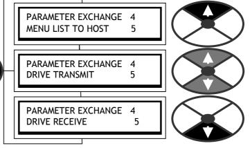
Transmitting parameters from the SPEDESTER to a host is defined as DRIVE TRANSMIT whereas receiving data by the SPEDESTER from a host is defined as DRIVE RECEIVE.
