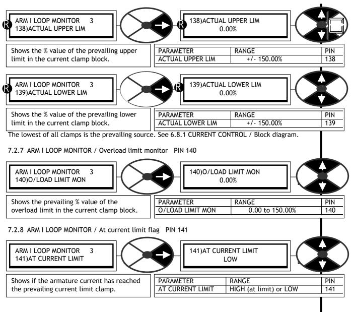
7.2.6 ARM I LOOP MONITOR / Actual prevailing upper/ lower current limits PINs 138 / 139
