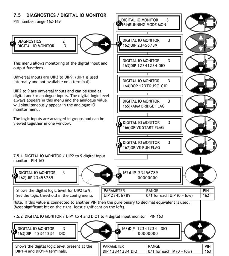
Note. If this value is connected to another PIN then the pure binary to decimal equivalent is used. (Most significant bit on the right, least significant on the left).
