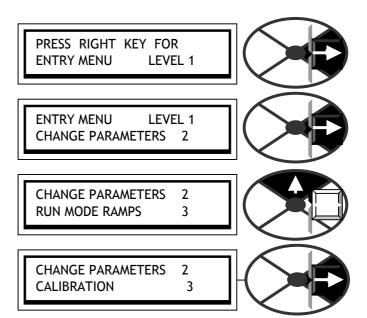
parameter adjustment window for each in turn. Modify each one to suit your system using the up/down keys. Use the left key to back out of each parameter adjustment window and return to the circular CALIBRATION menu.
