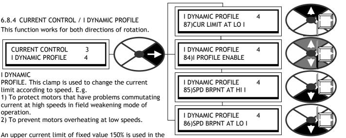
calculation. If 3)CURRENT LIMIT(%) is set lower than 150%, then 3)CURRENT LIMIT(%) will prevail. If current limits in the other current limit blocks are lower then they will prevail.
