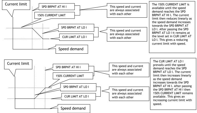
Note. The SPEED breakpoints may be set so that the profile starts low and goes high if required. If you try to bring the two speed breakpoints closer than within 10% of each other, then the higher speed breakpoint is internally assumed to be equal to the lower speed breakpoint + 10%.
