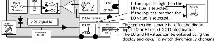
values, connect them using jumpers to the LO/HI value PINS. For logic only usage a value of 0.00% is read as a low. Any non zero +/- value is read as a high. Logic inversion is accomplished by entering 0.00% in the value for HI window and 0.01% in the value for LO window.
