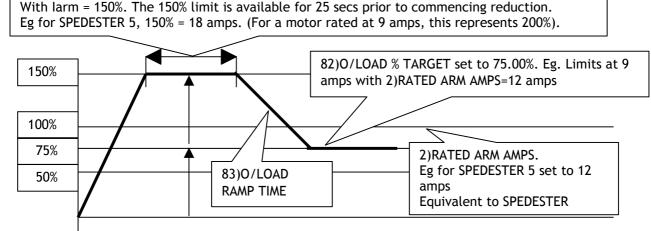
1) The current set on 2)RATED ARM AMPS (12 amps) represents 100% of the drive (SPEDESTER 5), but for this application must be deliberately set higher than the normal full load motor current (9 amps).
