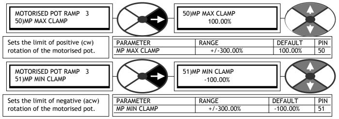
Note. Clockwise rotation is towards the +ve limit, anticlockwise rotation is towards the -ve limit. Always ensure the clamps allow some movement between them, do not let the clamps cross each other.
