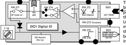
The connection is made here for the digital output block source. It may be a linear or logic value. After processing by the rectifier box it gets compared to the threshold. The comparator output state HIGH or LOW is then inverted or not inverted by the inverter mode box. It then proceeds to the output stage through the digital output enable switch and becomes a 24V logic signal. It is also available for internal connection. See 3.4.2 Digital inputs and outputs.
