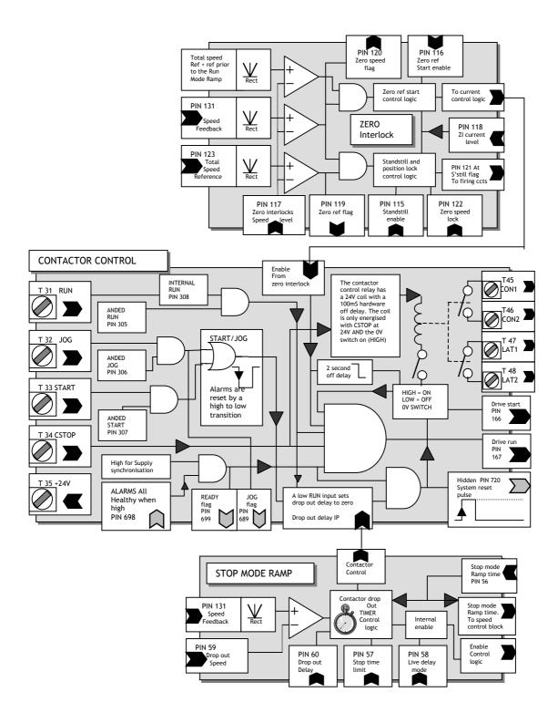
The following conditions must be true for the main contactor to be energised.
