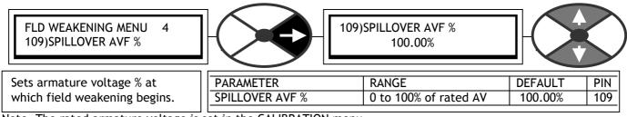
Note. The rated armature voltage is set in the CALIBRATION menu.
