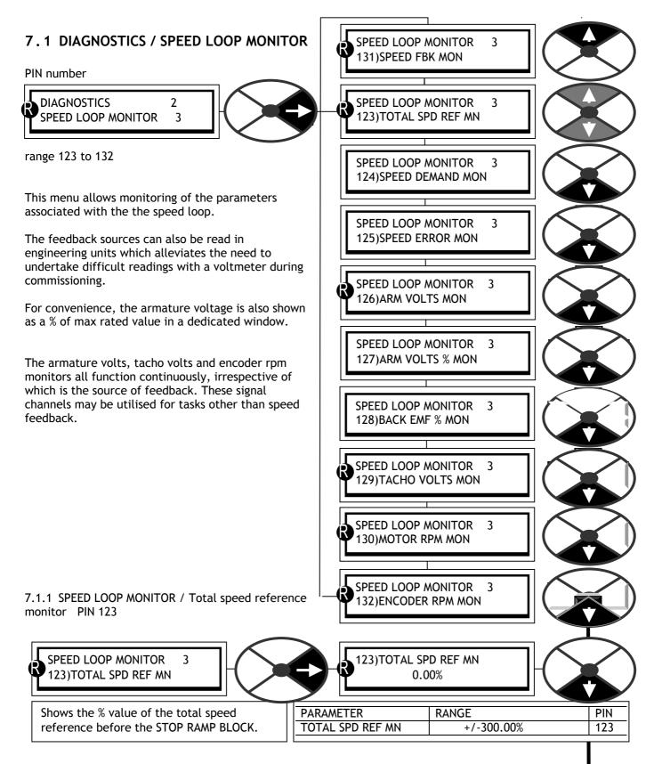
This parameter is a summation of all possible speed references including the RUN MODE RAMP. Note that the RUN MODE RAMP may be active when the unit is in stop mode. This feature allows cascaded systems to function even if a member of the system is stopped. See 6.2 CHANGE PARAMETERS / RUN MODE RAMPS.
