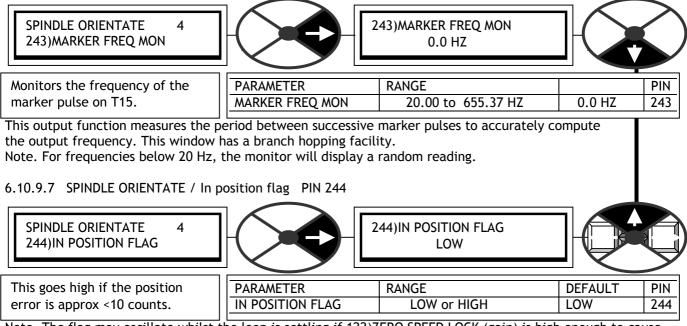
Note. The flag may oscillate whilst the loop is settling if 122)ZERO SPEED LOCK (gain) is high enough to cause overshoot. This window has a branch hopping facility.
