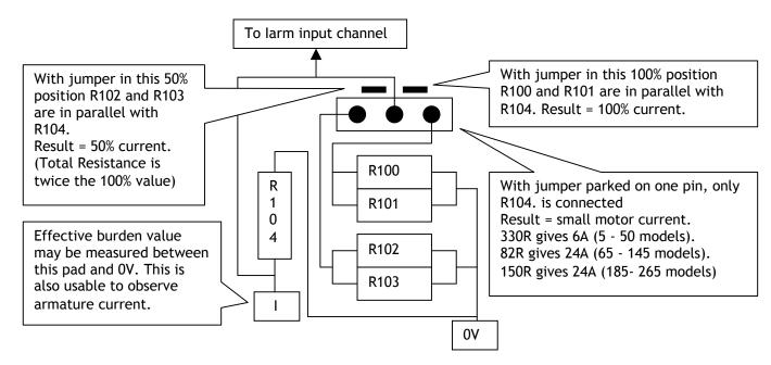
Note. After parameter 680) Iarm BURDEN OHMS has been altered, it will only apply after the following steps:-
