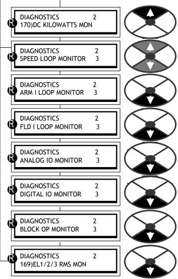
monitored. The UP key hops to the end of the branch above, and the DOWN key hops to the end of the branch below giving rapid access to the monitored parameters within each sub-menu. It also provides a reminder that you are not in a parameter changing menu, where this branch hopping feature is not available.
