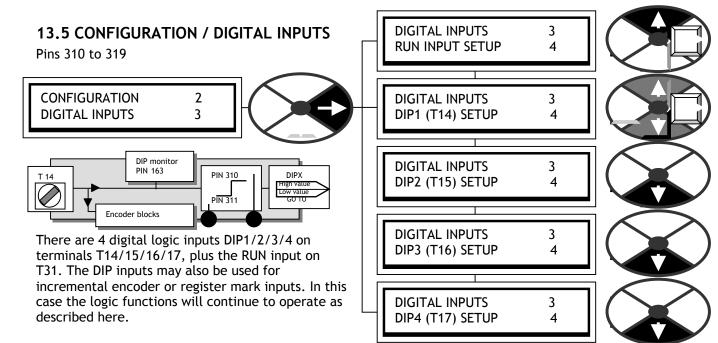
The LO and HI values can be entered using the display and keys, or may be connected to other output PINs using JUMPERS. This turns the function into a change-over switch for dynamic values. For logic only usage a value of 0.00% is read as a low. Any non zero +/- value is read as a high. Logic inversion is accomplished by entering 0.00% in the value for HI window and 0.01% in the value for LO window.
