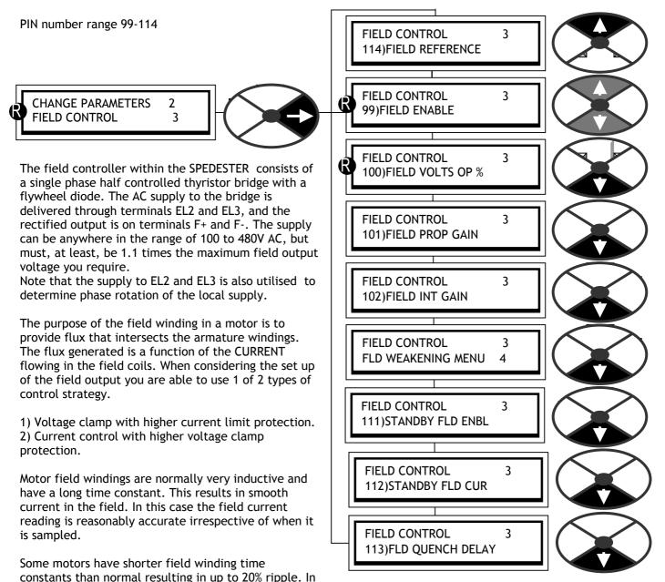
this case the SPEDESTER may sample the current at a non-ideal point in the cycle which will result in a slightly incorrect control level. (Usually no more than a few %) To normalise the field current back to its correct level it may be necessary to use the field current trim. See 6.1.12 CALIBRATION / Field current feedback trim PIN 15,
