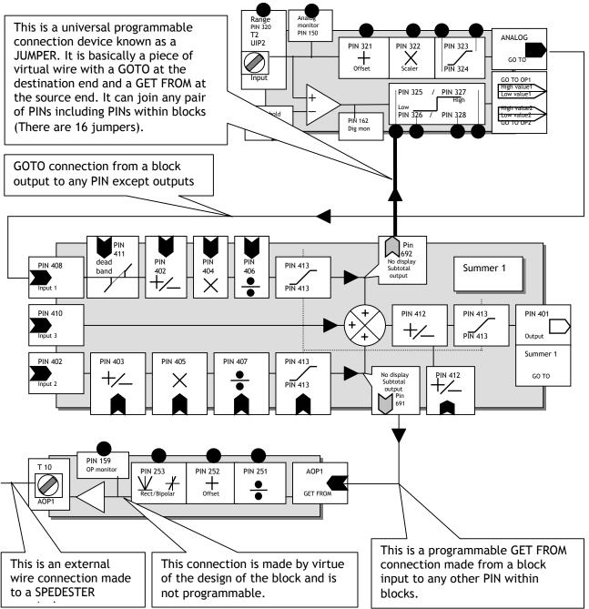
Note. To start a connection configuration session ENABLE GOTO, GETFROM must be set to ENABLED.
