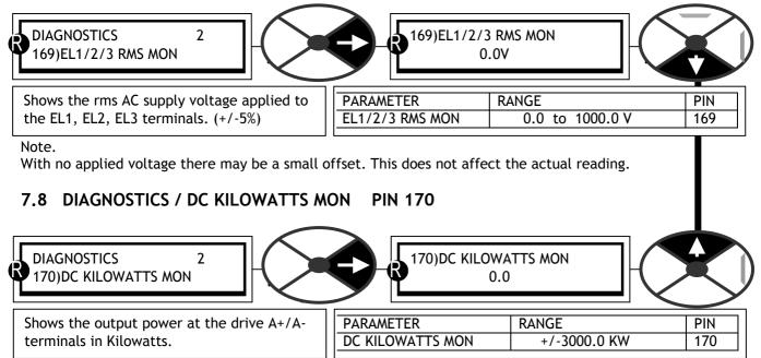
Note. A negative output power shows that the SPEDESTER is regenerating into the AC supply. The power available at the motor shaft will depend on the motor efficiency. (Typically 90 to 95%). To convert Kilowatts to Horsepower multiply by a scaling factor of 1.34.
