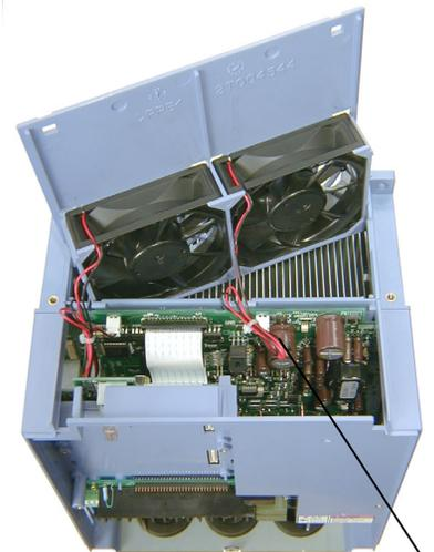
PWB connector for fan assembly wiring
