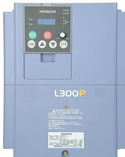
2. **Second-level access** - First, ensure no power source of any kind is connected to the inverter. If power has been connected, wait five minutes after powerdown and verify the Charge Lamp indicator is OFF to proceed. Then locate the recessed retention screw at the bottom of the main front panel. Use a small Phillips screwdriver to remove the screw. Press the two latch release areas near the “L300P” label as shown, and simultaneously slide the lower front downward to release for removal.
