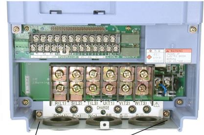
Retention screws for wire entry plate
